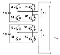
Fig-5 Block diagram of 5-level CHB inverter model
