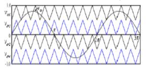
Fig 7 level shifted phase shifted carrier pwm
