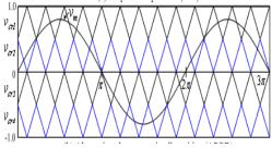
Fig-8 Alternative phase opposite disposition (APOD)
